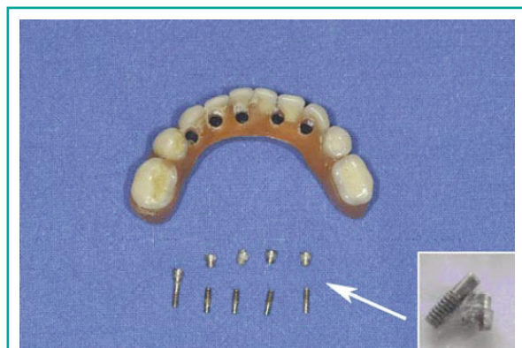
Figure 3 The passant screws broken after the masticatory cycle.
