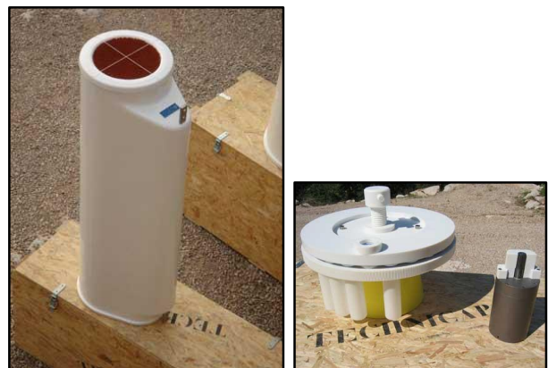
Figura 6. Technicap Sediment trap
