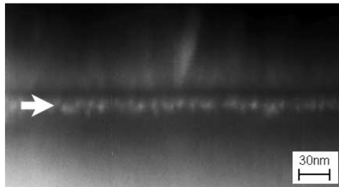
Fig. 4. – STEM dark-field image of the Sb-implanted Si specimen. The implanted Sb segregated in small precipitates about 20 nm below the surface. The arrow marks the position of the precipitates.
