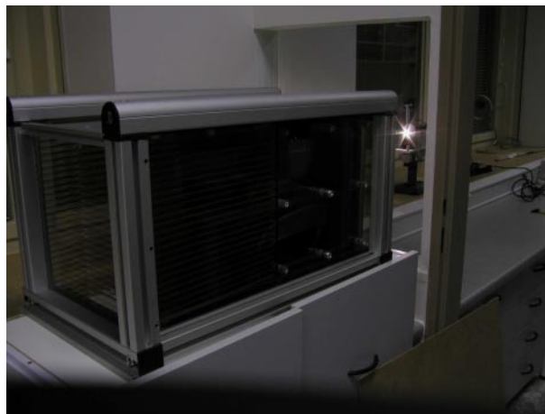
Fig. 1. – The large Lobster-Eye telescope prototype ( 300 \times 300 mm plates, Schmidt arrangement) represents the largest Lobster telescope test module constructed so far.
