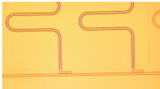
Fig. 12. – Microwave resonators coupled to a CPW line.
