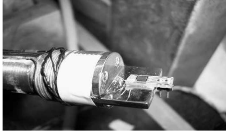
Fig. 1. – Cold-finger liquid-nitrogen cryostat and SiPM-thermometer glued.
