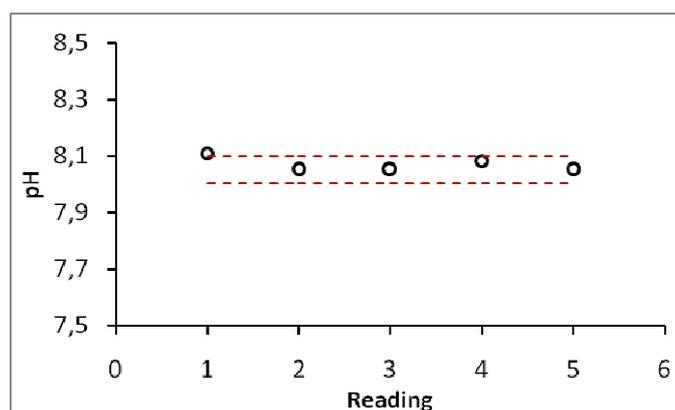
**Fig. 8. pH calculated in 5 consecutive scans in sea water (in Oristano) as compared with the range of pH indicated by the reference pH meter (between 8.0 and 8.1).**
