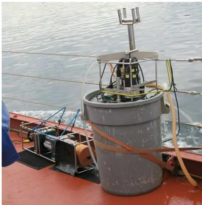
**Fig. 11. CTD on the Oceania deck measuring surface pumped water underway**
