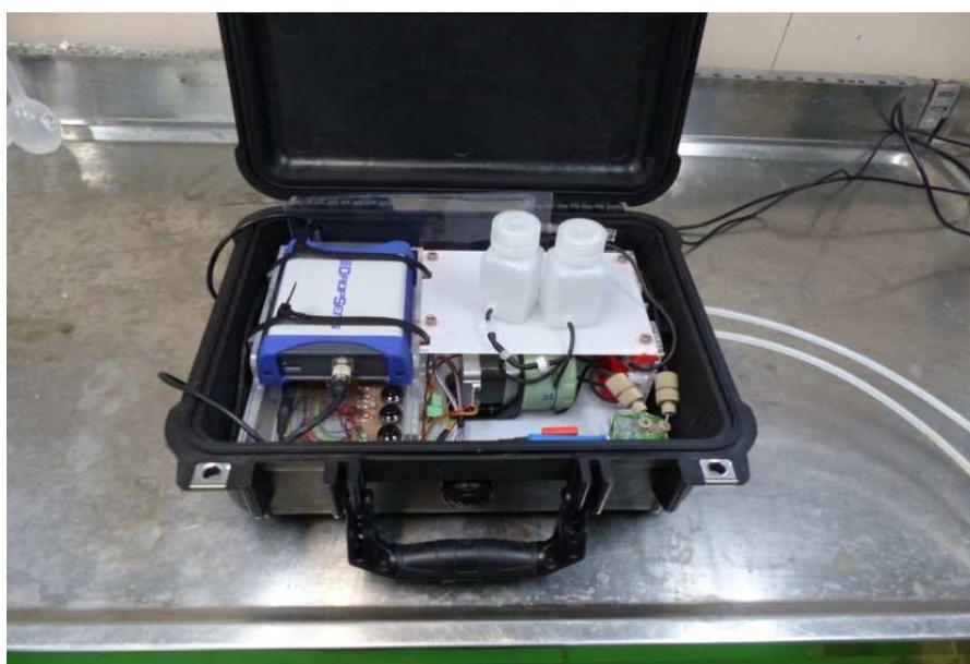
**Fig. 45. Heavy Metals System Gen 1 on-board the RV Minerva Uno**
