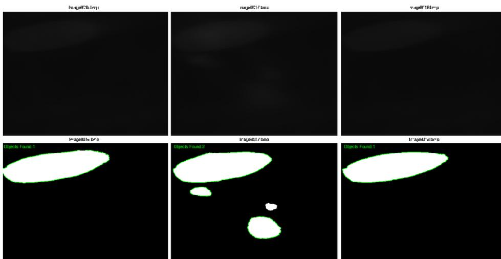
**Fig. 33. Detected microplastics (Real image—up /Processed image—below)**
