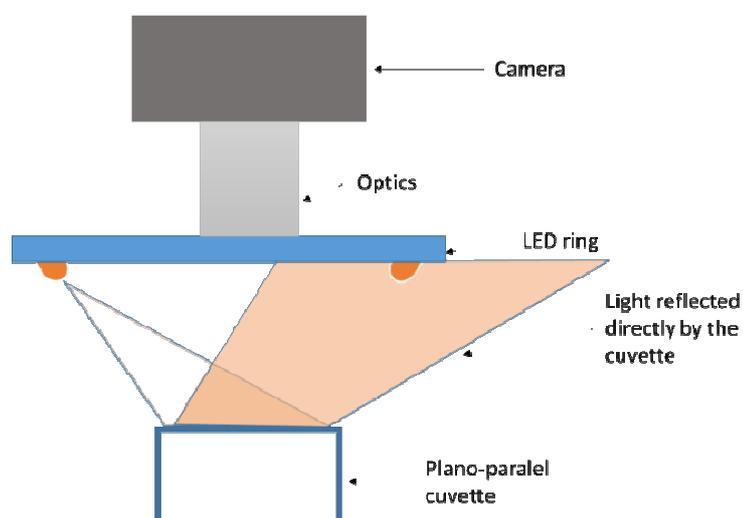
**Fig. 44. Schematic representation of the suggested modification (with a plane-parallel cuvette and properly diaphragmed illumination)**
