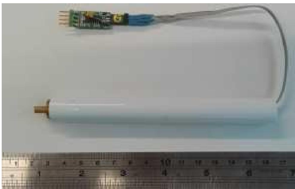
**Fig. 1. New housing for temperature sensor attached to the Tyndall PCB**
