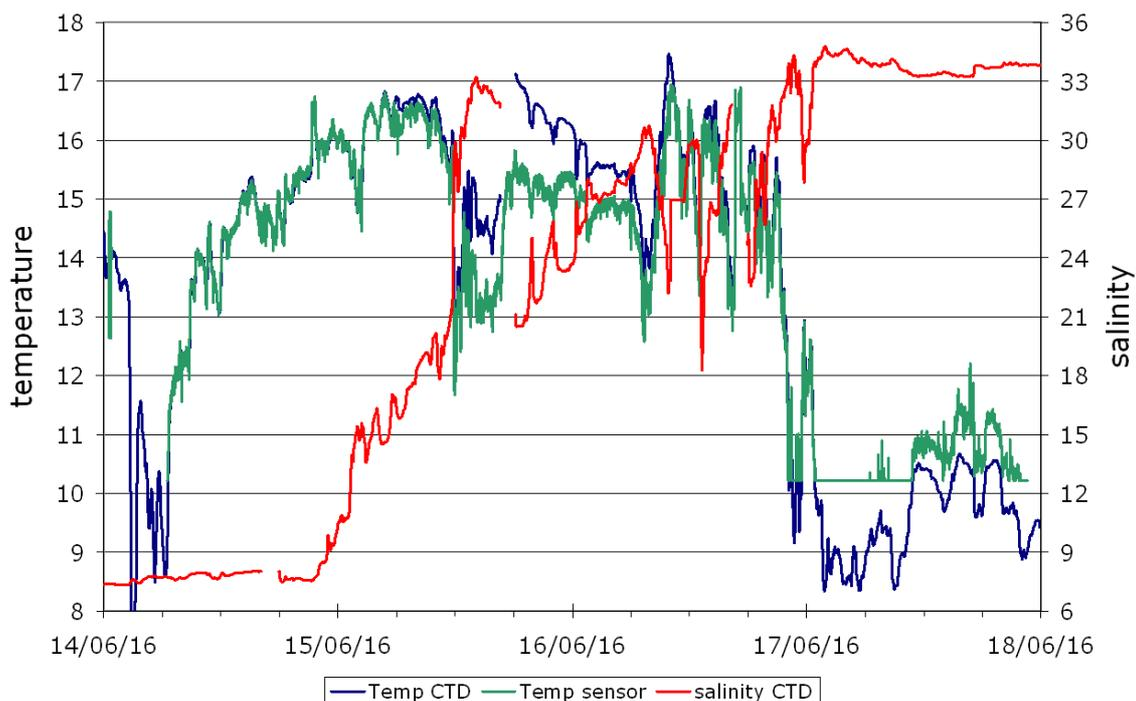
**Fig. 12. Four days time-series of temperature from CTD and new sensor, and salinity from CTD underway the Oceania course up to 00:00 18/06**
