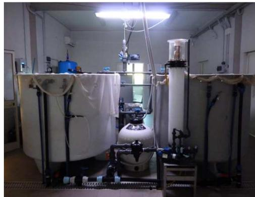
**Fig. 56. The tanks available at IAMC CNR in Oristano for experiments: 2300 l (left) and 900 l (right)**
