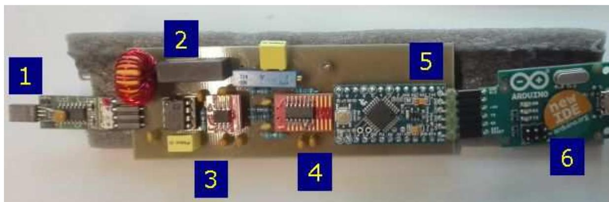
**Fig. 7. Complete board used to connect the sensor and deliver a digital code through a USB. Tyndall PCB conditioner (1) to sensor including a 100 nF capacitor, DC/DC 5 to 12 V converter (2), reference voltage (3), MPC 3424 A/D converter (4), Arduino microprocessor (5) and USB serial converter (6) to computer**
