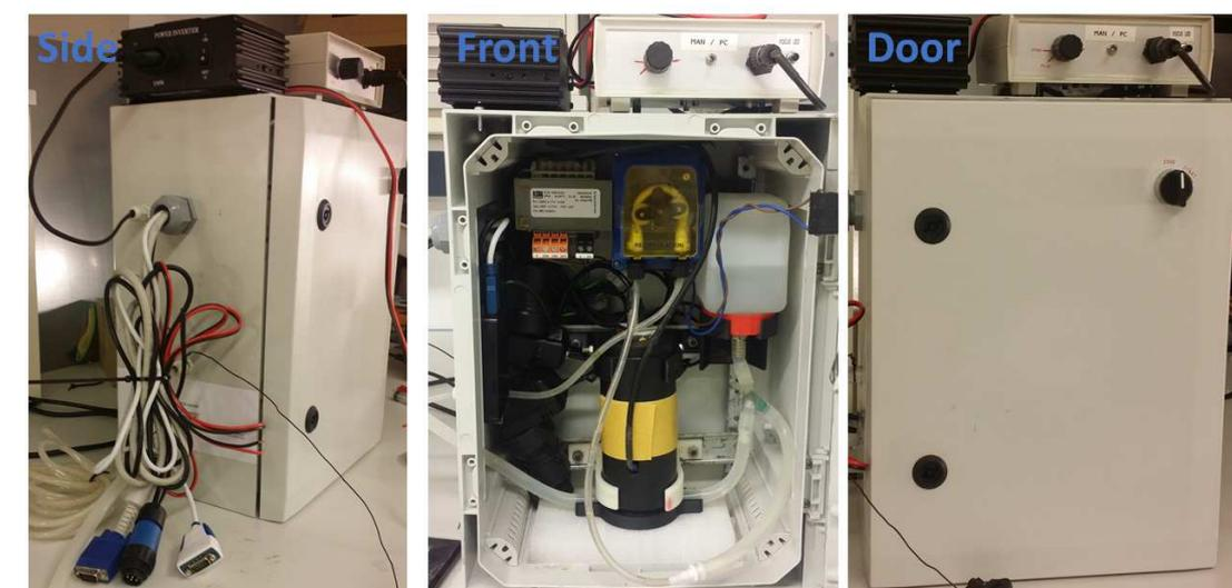
Fig. 27. Second functional prototype of microplastic sensor
