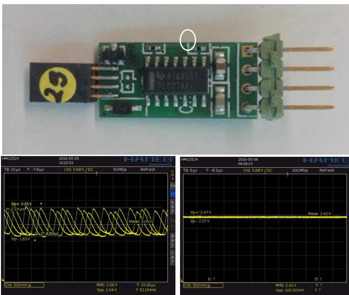
**Fig 6. a) PCB conditioner (top), b) direct output from sensor+PCB shown by the oscilloscope (left) and c) the same output corrected with a 100nF capacitor (right)**
