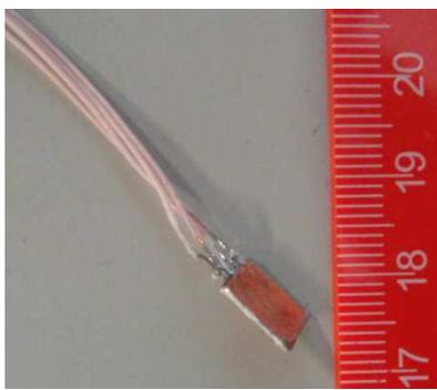
**Fig. 2. Temperature sensing device. The sensing element is located inside the copper housing. Four wires coming out from the sensor for electrical measurements (scale is in cm)**
