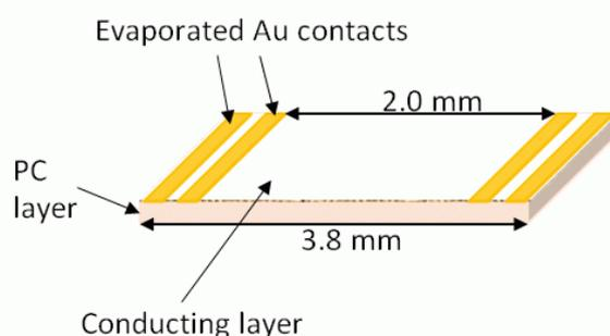
**Fig. 3. Sketch of the four Au contacts, evaporated over a conducting surface of the BL film. Thickness of the evaporated contacts was 100 nm of Au plus 10 nm of adhesive layer of Cr. The width of the contacts was 150 nm**
