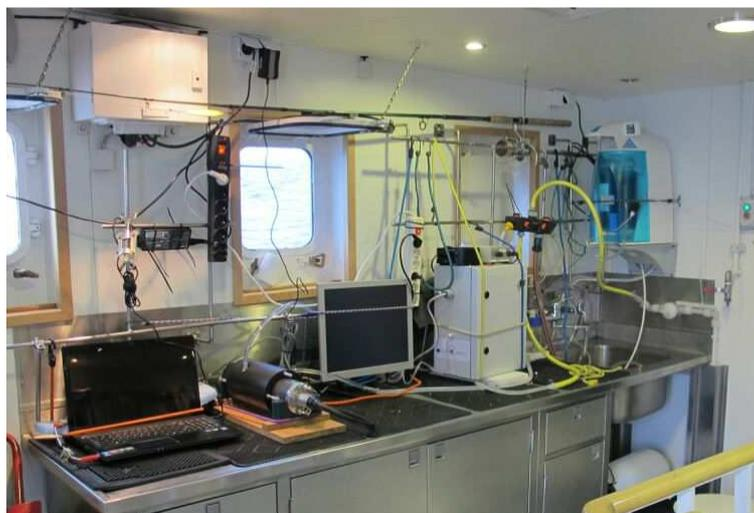
**Fig. 10. Instruments using surface pumped water underway at the Oceania wet laboratory**
