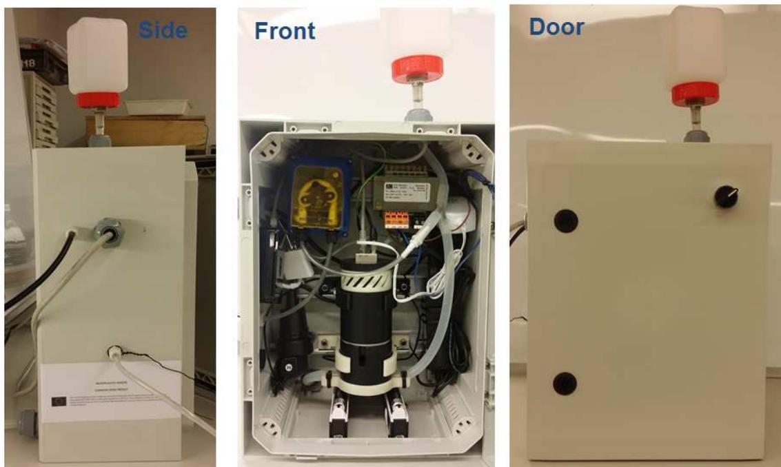
Fig. 26. First functional prototype of microplastic sensor
