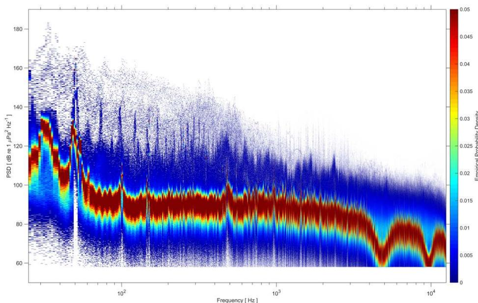
**Fig. 54. Spectral probability density of recorder deployment data from 28-29 September 2016. Data are presented with 1-Hz frequency resolution.**
