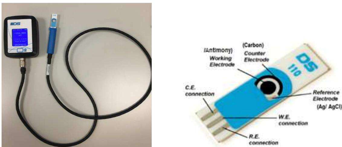
**Fig. 3. (a) Potentiostat, connector and screen printed electrode; (b) Antimony screen printed electrode**
