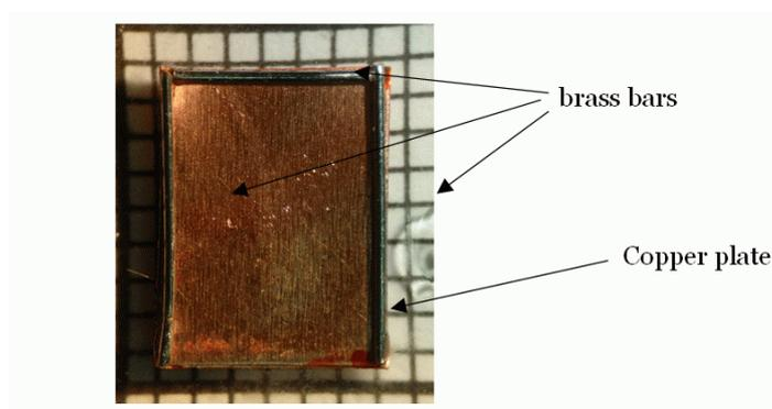
**Fig. 5. Inside the housing of the sensor**
