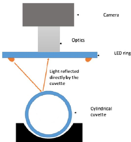
**Fig. 43. Schematic drawing of the current prototype configuration**
