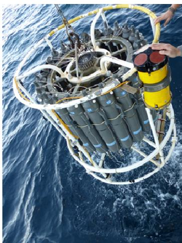
**Fig. 16. General Oceanics Rosette Sampler**
