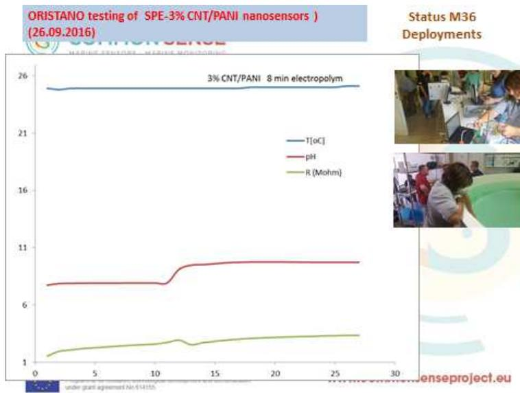
Fig. 5 (above) and 6 (below). Field testing at CNR in Oristano, September 2016 with resistivity [kΩ] on abscissas and time [minutes] in ordinates
