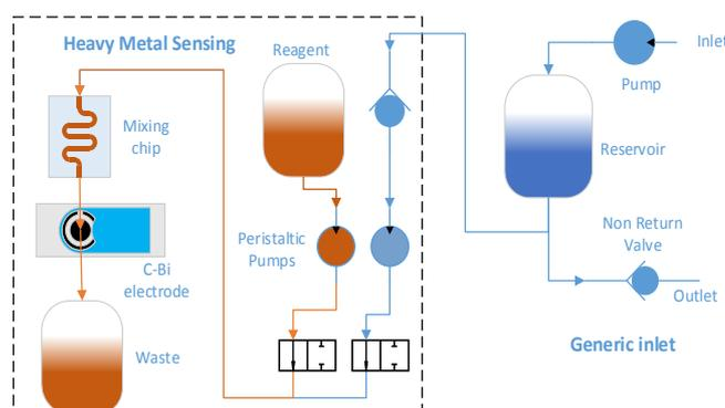
**Fig. 46. Fluid schematic of the version 2 heavy metal system**
