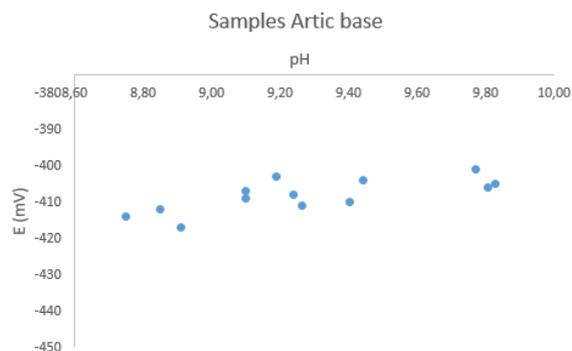
**Fig. 10. Mean potential recorded vs pH values: Arctic-June 2016**
