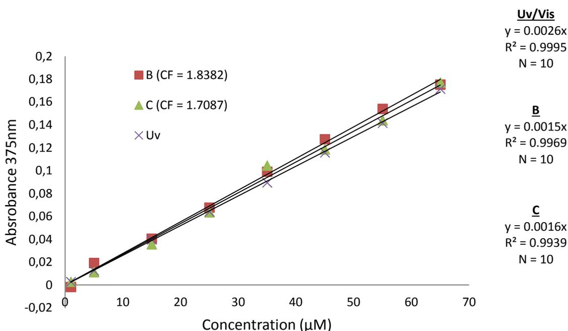
**Fig. 11. Inter-laboratory results obtained using Phosphate standards provided by Tellab (1-65µM). The graph shows the comparison of the UV-Vis benchtop system (UV-Vis) the COMMONSENSE benchtop system B and C**
