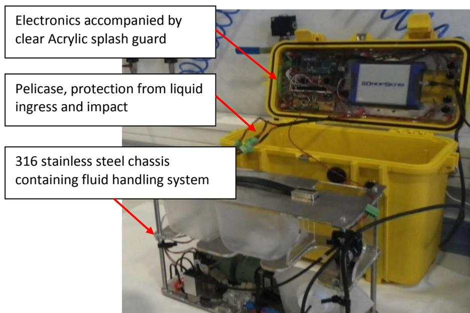
**Fig. 47. Heavy Metals System Gen 2: New fluidic design incorporated into a Pelicase waterproof housing and 316 stainless steel internal chassis**
