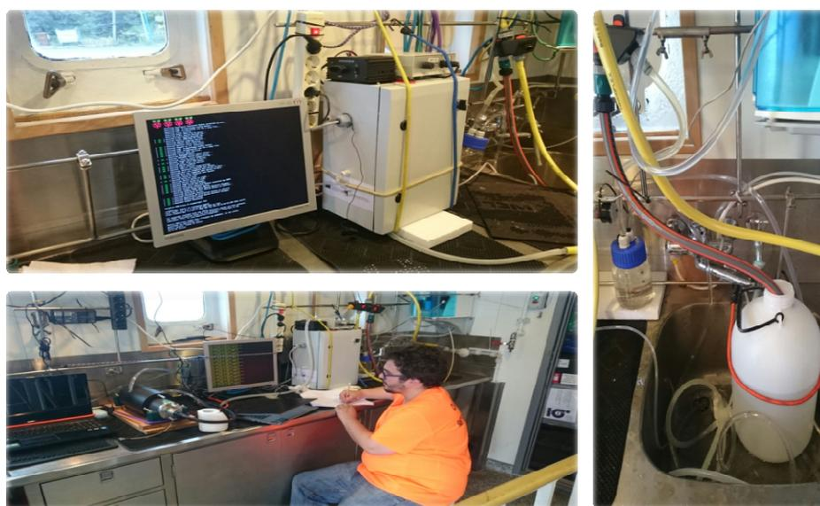
**Fig. 35. Set-up of microplastics sensor inside the OCEANIA research vessel**
