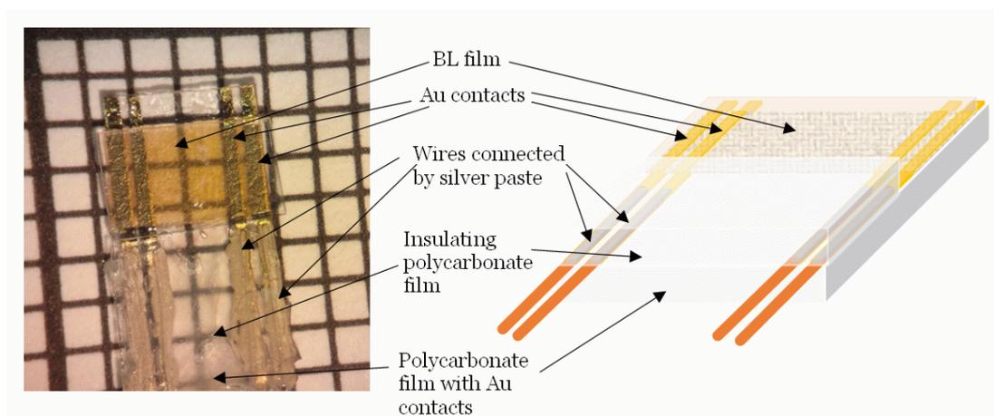
**Fig. 4. Electrical contacts with BL film and its insulation from the housing: (left) photo image, (right) schematic view**
