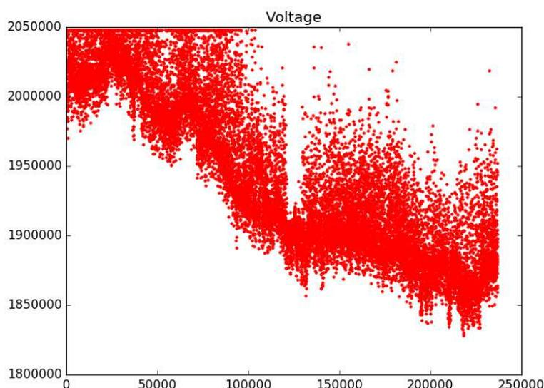
**Fig. 14. Time series (sec) of sensor output ( $\mu\text{V}$ ) in an attempt to reproduce a progressive temperature increase in laboratory conditions after the cruise**
