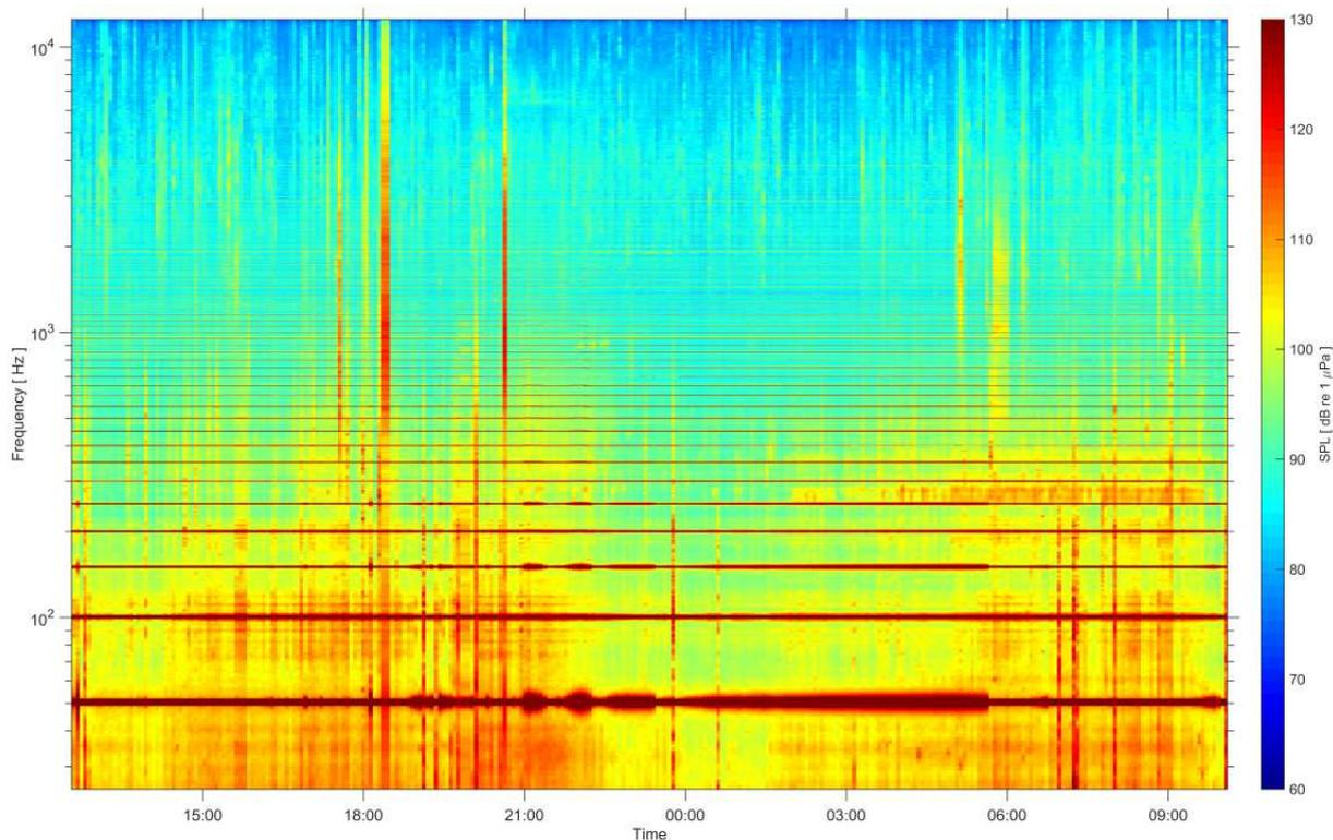
**Fig. 53. Power spectral density of recorder deployment data from 28-29 September 2016. Data are at 1-Hz frequency resolution, presented as 60-s averages**
