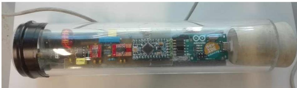
**Fig. 8. Sensing electronics encapsulated in a methacrylate tube.**
