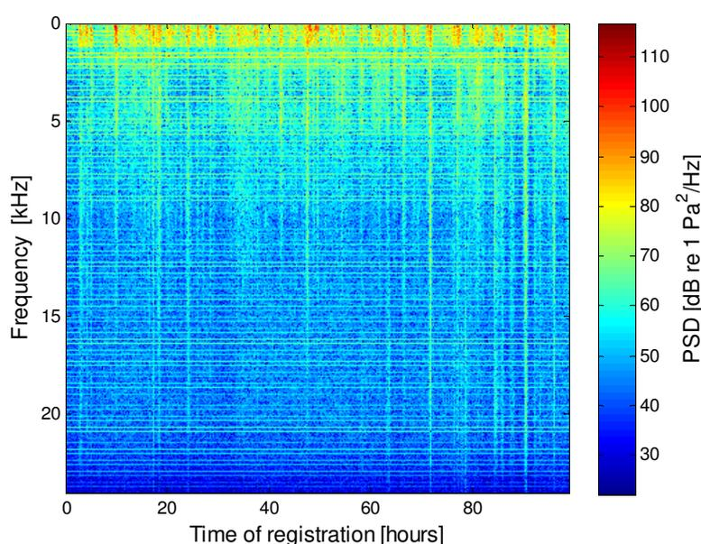
**Fig. 52. Spectra of signals registered by commercial buoy, with low sensitive hydrophone.**
