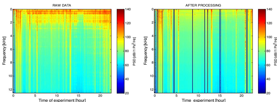
**Fig. 51. Power Spectra Density Level of underwater noise before (on the left) and after removing signals with the local disturbances (on the right).**
