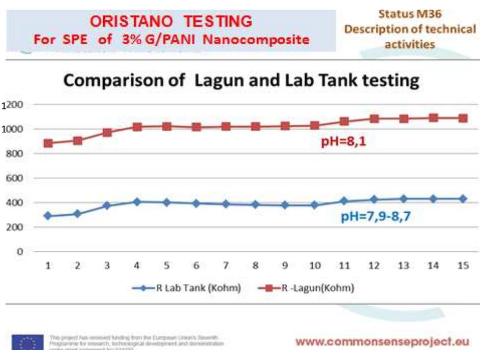
**Fig. 7. Comparison of lagoon and Lab-tank testing with resistivity [k $\Omega$ ] on abscissas and time [minutes] in ordinates**
