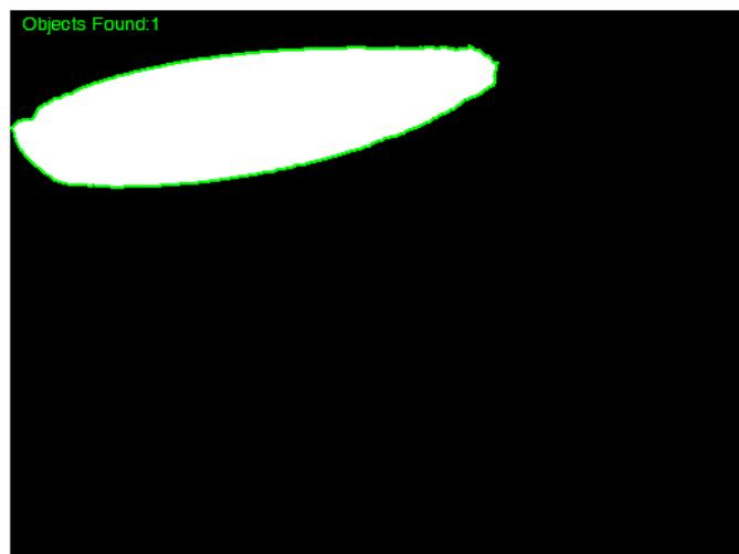
**Fig. 5. Wrongly identified object due to stray reflection on the cuvette surface**
