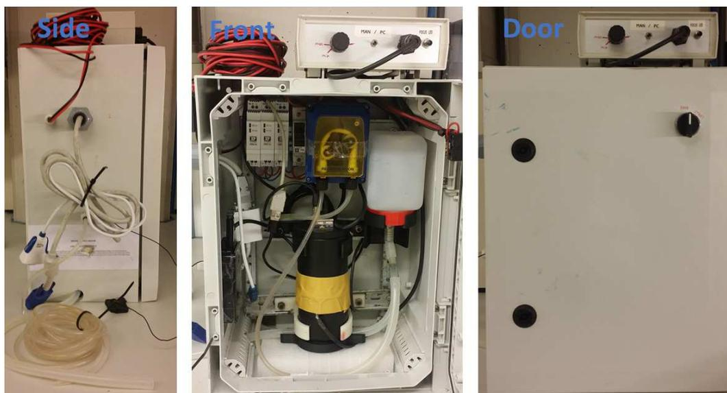
Fig. 28. Vendée Globe version of microplastic sensor
