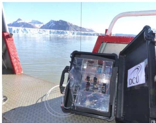
**Fig. 25. Deployable CS nutrient sensor acquiring samples from Kronebreen Kongvegen glacier**
