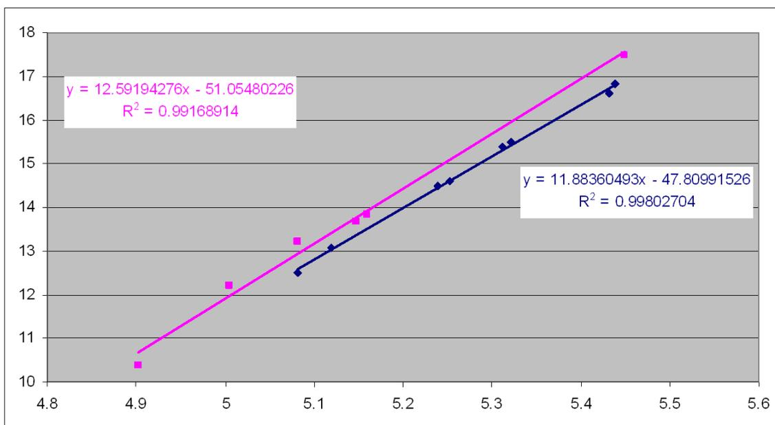
**Fig. 13. Linear adjustment of sensor output converted to conductivity ( $\mu\text{S}$ ) and CTD temperature. Blue dots (rightmost line) correspond to the first period (roughly before noon 15 June) and pink dots (left) to the second period (see fig. 12)**
