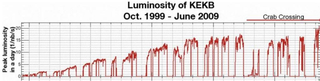
Fig. 1. – Daily peak luminosity of the KEKB collider.
