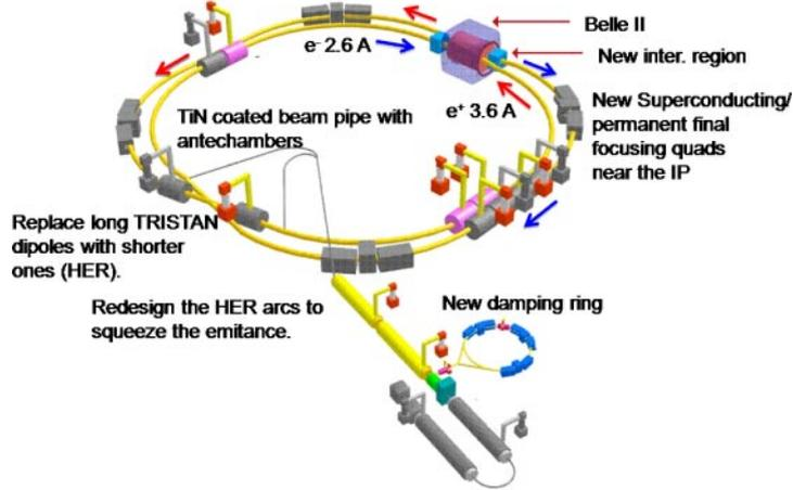
Fig. 2. – The main parts of the KEKB upgrade.
