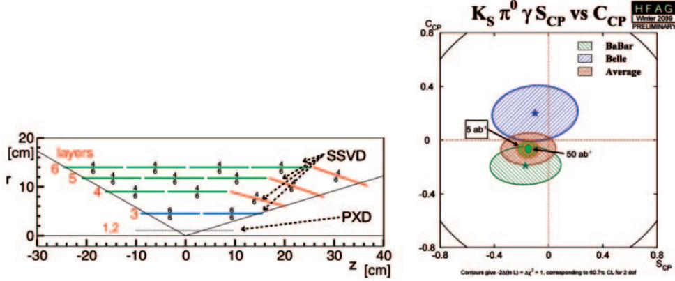
Fig. 5. – Left: A schematic view of the upgraded semiconductor detector. Right: Comparison of the current [10] and expected precision on direct and indirect  $CPV$  in  $B^0 \rightarrow K_S \pi^0 \gamma$ .
