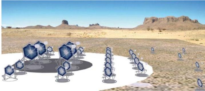
Fig. 1. – Possible layout of the composite CTA southern observatory. The area covered amounts from 1 to 10 km<sup>2</sup>. This particular configuration corresponds to four Large Size Telescopes (LST) at the center of the array surrounded by about thirty Middle Size Telescopes (MST) and an extended crown of Small Size Telescopes (SST).
