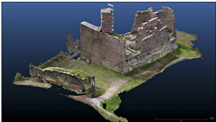
Fig. 3 – Screenshot of the photogrammetric model of castle Hohenecken in CloudCompare.
