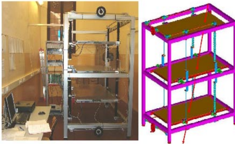
Fig. 2. – The EEE muon telescope: 3 MRPCs with the mechanical structure. The moving equipment allows to vary the distance between the chambers.
