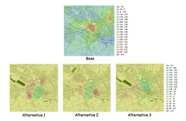
Fig. 8. Example of urban metabolism analysis conducted in the BRIDGE project. Mean surface runoff (mm h<sup>-1</sup>) for summertime for the Firenze study case. The alternative scenarios (bottom) are evaluated as runoff difference with respect to the base case (top)
