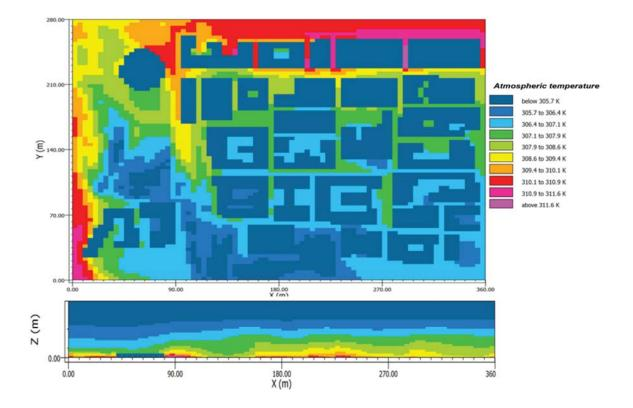
Fig. 3. Atmospheric temperature in a green scenario simulated with ENVI-met model, historical city center of Teramo, Italy
