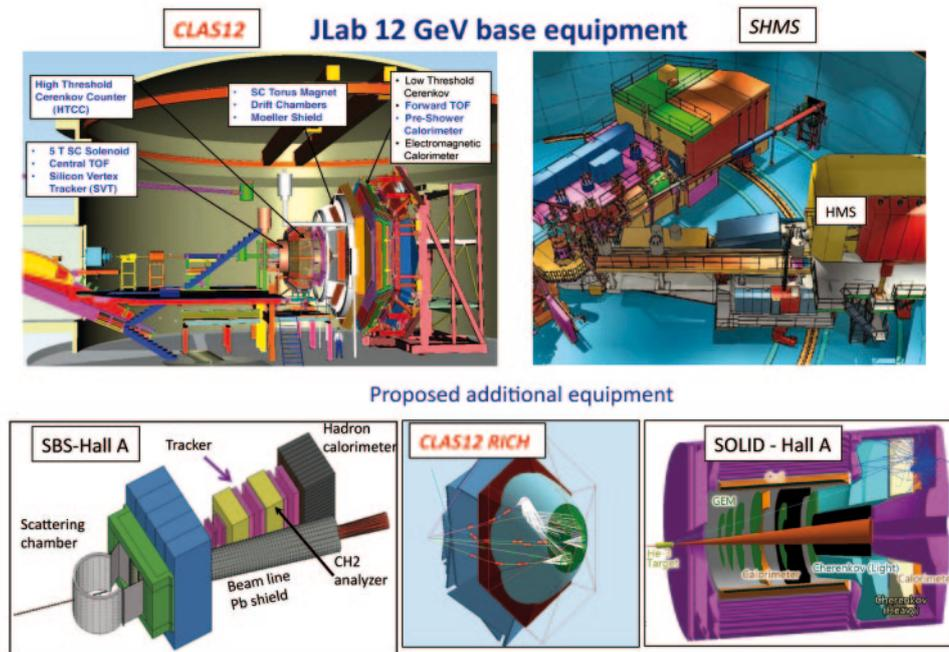
Fig. 2. – Experimental equipment to support the multi-dimensional nucleon structure program at the JLab 12 GeV upgrade.
