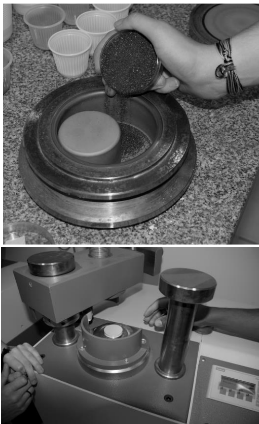
Figure 6. Crushed sample (left) and detail of the sample exit (right).
