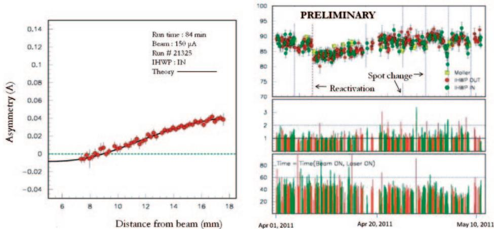
Fig. 2. – The measured Compton asymmetry (left). The measured polarization as a function of time (right, top). The dashed and dotted lines represent various events such as reactivation and change of spot in the photo-cathode of the polarized electron source. The error bars represent the statistical and preliminary systematic uncertainty added in quadrature. The value of the statistical uncertainty (right, middle) and the time interval of each data point (right, bottom) is also shown.
