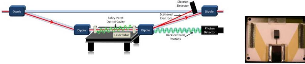
Fig. 1. – Compton polarimeter layout (left) and the diamond micro-strip detector (right).
