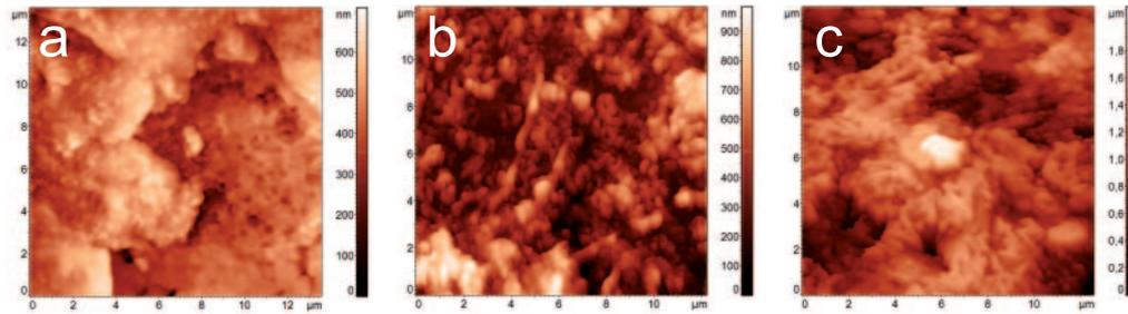
Fig. 1. – AFM images of: (a) uncoated GB; (b) SWCNTs-coated GB and (c) *Streptococcus mutans* colonized SWCNTs-coated GB.
