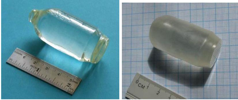
Fig. 4. – Boule (left) and scintillating element (right) of  $^{106}\text{CdWO}_4$  crystal grown by the low-thermal-gradient Czochralski process used by the DAMA collaboration for the experiment on the double beta decay of  $^{106}\text{Cd}$  isotope.
