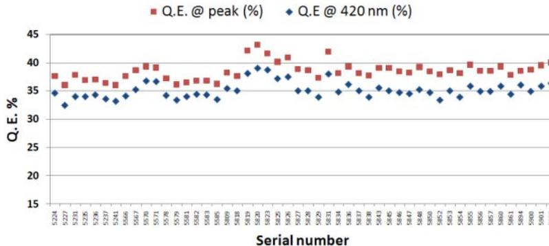
Fig. 1. – Quantum efficiency at peak and at 420 nm of each one of the 50 high Q.E. PMTs, installed in DAMA/LIBRA-phase2 [16].
