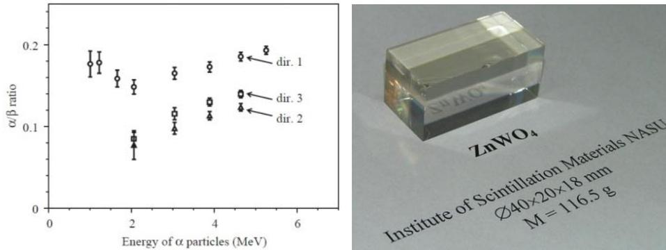
Fig. 10. – ADAMO project. Left: dependence of the  $\alpha/\beta$  ratio on energy of  $\alpha$  particles measured with  $\text{ZnWO}_4$  scintillator for different  $\alpha$  directions of irradiation. The anisotropic behaviour of the crystal is evident. Right: a picture of a  $\text{ZnWO}_4$  scintillator.
