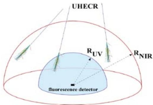
Fig. 6. – Conceptual idea of NIRFE: NIR fluorescence has much longer absorption length in air than UV. Hence an increase of the observable event rate is expected.
