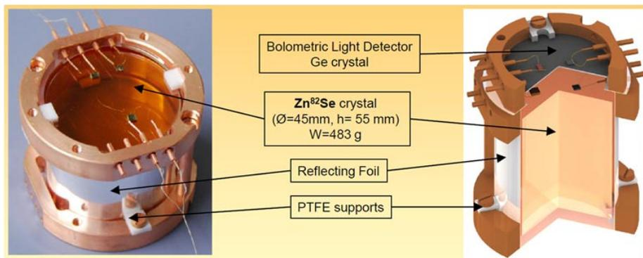
Fig. 9. – Photo and schema of a typical detector of Lucifer experiment.
