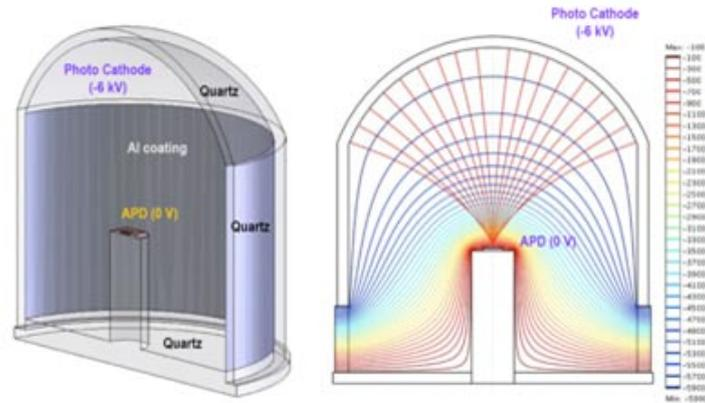
Fig. 2. – Schematic views of the QUPIDs, implemented for light read-out in Liquid Noble gases detectors.
