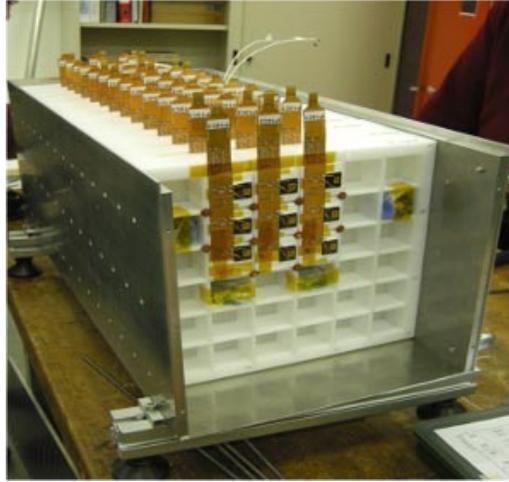
Fig. 5. – A photo of the GAMMA400 prototype tested on an ion beam at CERN.
