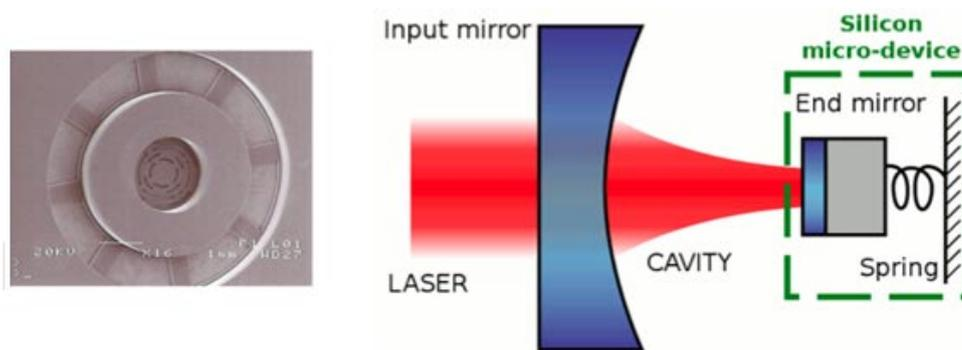
Fig. 7. – MEMS mirrors for quantum opto-mechanics. Radiation pressure couples a moving mirror and laser light in a Fabry-Perot cavity.
