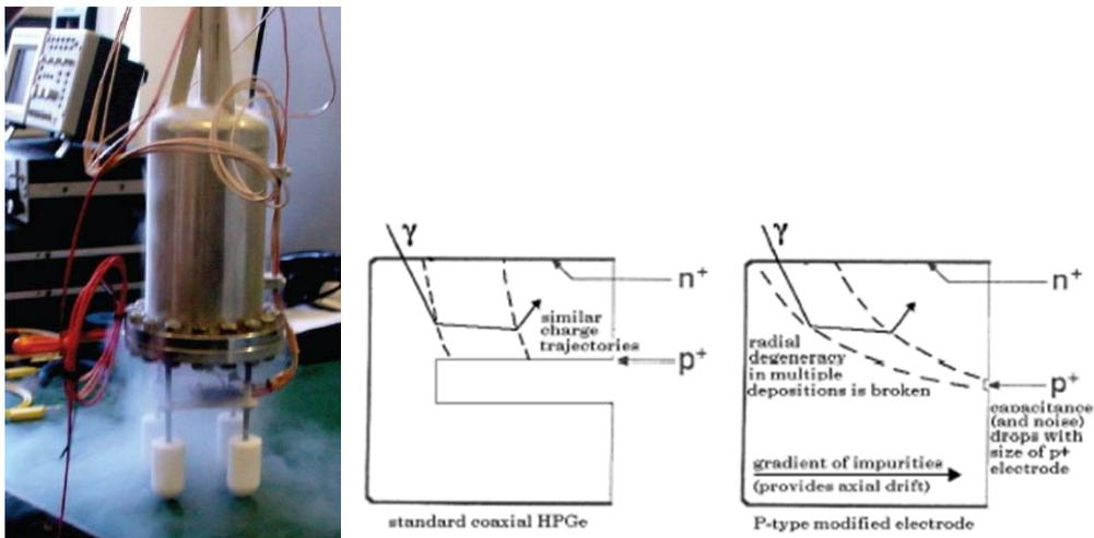
Fig. 3. – A photo of a HPGe detector of GERDA and the conceptual difference between HPGe and BEGe detectors.
