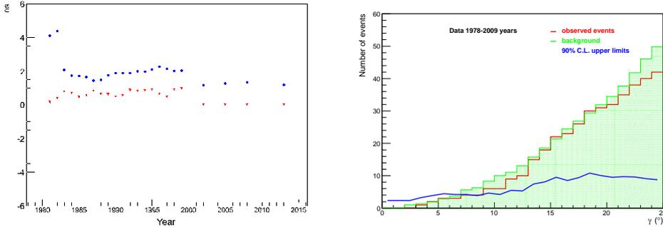
Fig. 1. – Left: measured mean (red) and sigma (blue) values of PMTs time off-set distributions over all 3150 counters of the BUST since December of 1978 till January of 2013. Right: the 90% C.L. upper limits on signal events in the direction toward the Sun (blue) in cone half-angle  $\gamma$ . Measured (red) and background (green) events are also shown depending on the value of  $\gamma$ .
