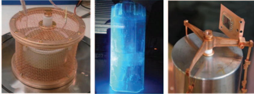
Fig. 5. – The three different options for the mini-shroud around the Ge detector strings: (a) the meshed Cu mini-shroud; (b) the nylon mini-shroud; (c) the BEGe detector with the SiPM. In this last case both the detector and the SiPM are enclosed by the Cu mini-shroud from Phase I.
