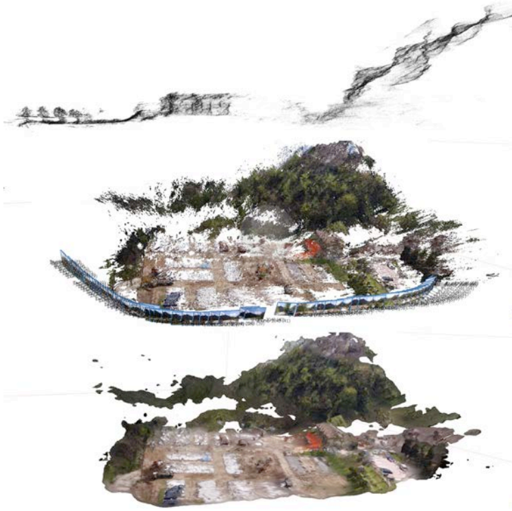
Fig. 3 Arquata del Tronto case study. From top-down: section of the 3D point cloud; point cloud with aligned photos; meshed model
