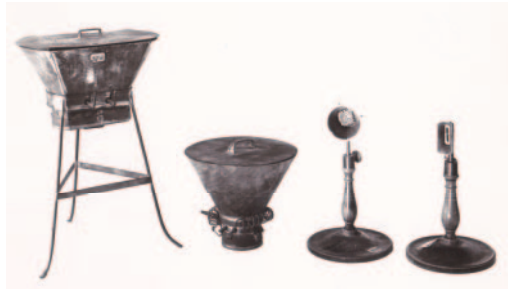
Fig. 2. – Thermopiles constructed and employed by Melloni. From the left, thermopile with 14, 16, 25 and 10 elements. Macedonio Melloni Collection of Physics. Photo Vaghi 1954.
