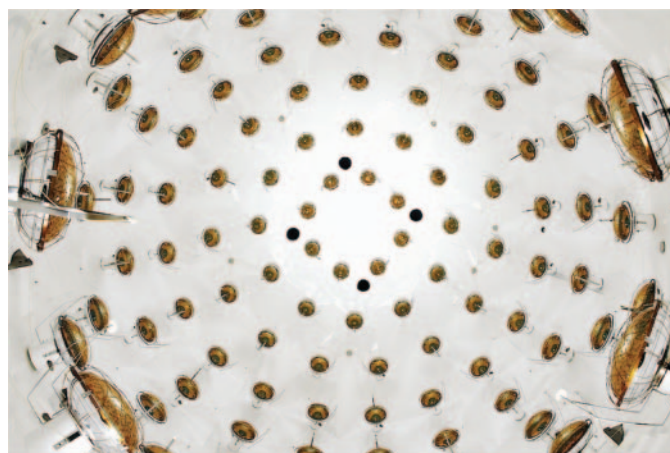
Fig. 2. – Internal view of the neutron detector from its top port.
