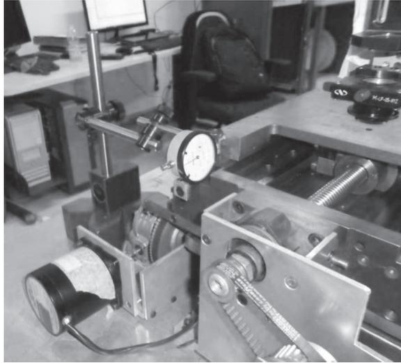
Fig. 10. – Comparator mounted on one of the two side of the motorized plane.
