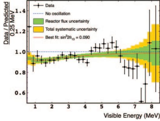
Fig. 5. – Data/predicted spectrum. The best fit is shown in red whereas in dashed blue it is shown the expectation in case of no oscillation, *i.e.*  $\theta_{13} = 0$ .
