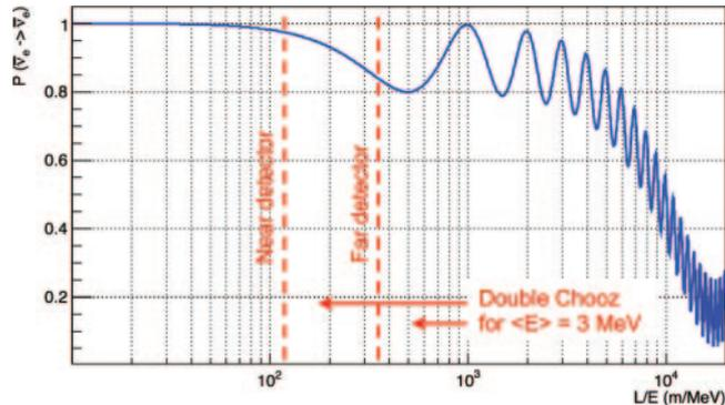
Fig. 1. – Oscillation probability  $P(\bar{\nu}_e \rightarrow \bar{\nu}_e)$  as a function of  $L/E$ . The regions covered by the near and the far detector are shown by the red dashed lines.
