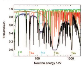
Fig. 1. — Transmission through a blind sample with the composition given in table I. The experimental transmission is compared with the result of a RSA. The contribution due to the different elements present in the sample is also shown.
