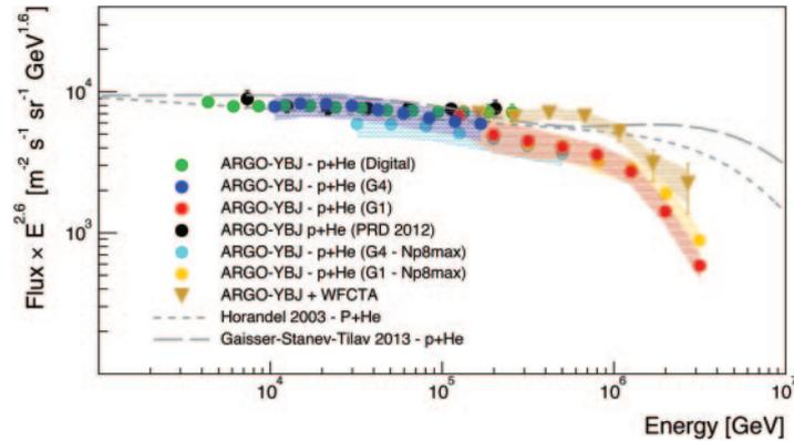
Fig. 3. – Cosmic ray proton plus helium spectrum measured by ARGO-YBJ. Results of the digital data (green) [8], Analog data with the bayesian technique (red and blue), Analog data with event-by-event energy reconstruction (light blue and yellow) [4] and Hybrid (brown) [5] analyses are reported. The curves of the proton plus helium spectrum according to the Hörandel [11] and GST [12] models are also shown.
