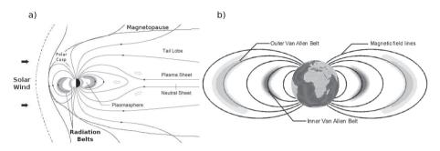
Fig. 1. - (a) Schematic representation of the Earth's magnetosphere in the meridian plane (figure redrawn from https://ase.tufts.edu/cosmos/). In this figure the Sun is on the left side. (b) Schematic representation of the inner and outer Van Allen radiation belts (figure redrawn from http://www.nasa.gov/).
