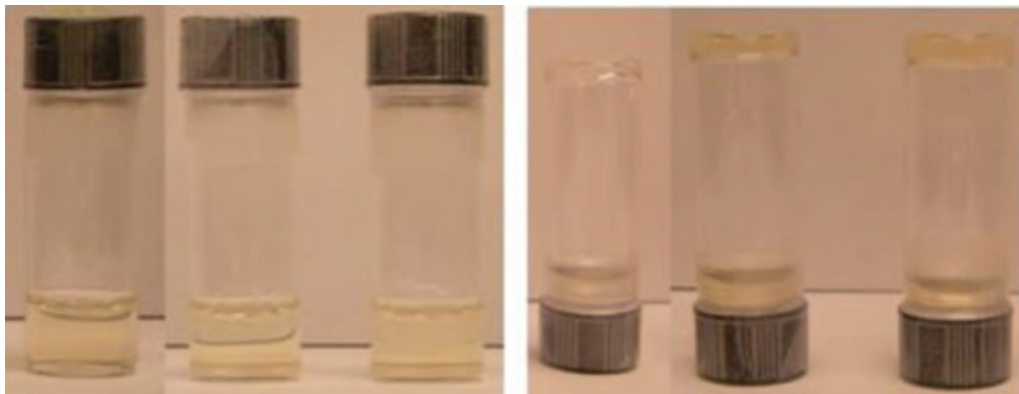
Fig. 6. – The gelation of \phi = 15\% in critical- and near-critical-concentration lutidine. Left: the solvent mixture is shown; right: we put the bottle upside down and then we can see gelled solid phase at the bottom of the bottles clearly. Lutidine concentration c_l from left to right is 29 wt%, 31 wt% and 33 wt%, respectively.
