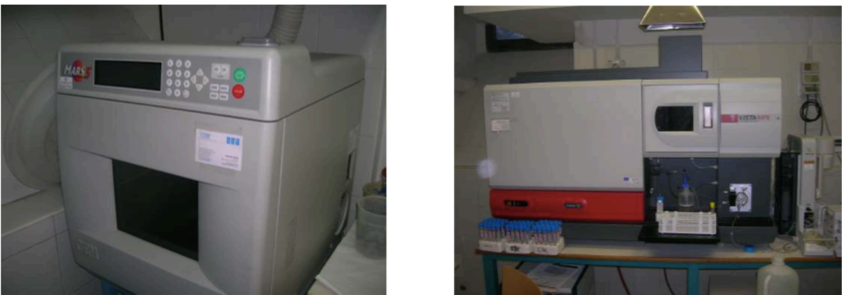
Figure 2: microwave oven CEM MARS-5 and ICP-AES Varian Vista MPX used for Cd and As determination.
