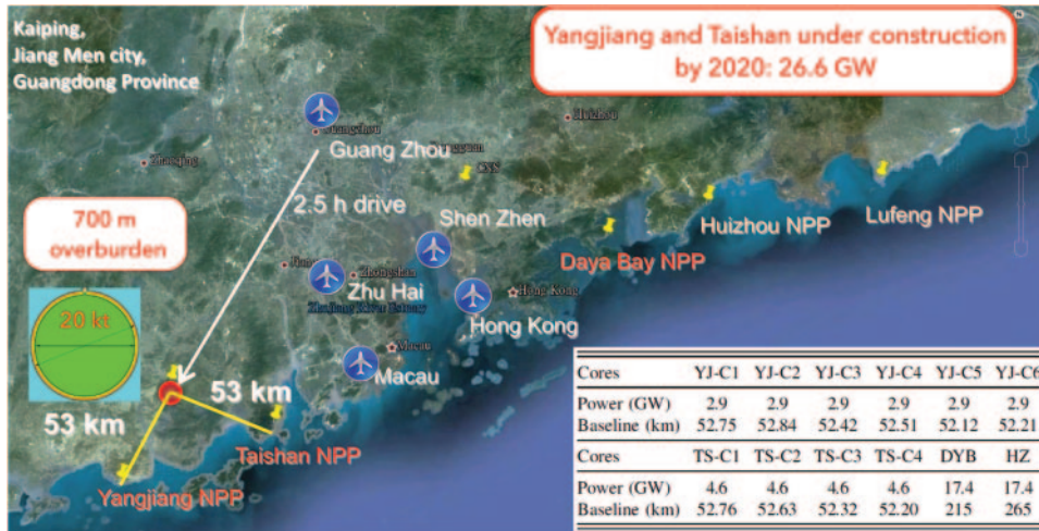
Fig. 1. – Location of the JUNO site. The distances to the nearby Yangjiang and Taishan nuclear power plants are both 53 km. Daya Bay nuclear power plant is 215 km away. In the inset the power and distance of the different cores from the detector are stated. The two of the four cores of Taishan nuclear power plant have been planned by the company, but the approval by the government is pending.
