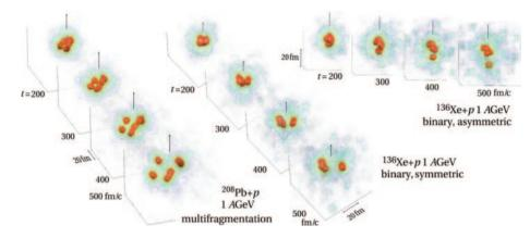
Fig. 4. – Spallation events followed in configuration space and producing fragments through a process of fragmentation and partial reaggregation.
