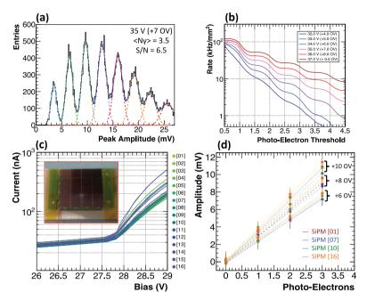
Fig. 1. – (a) Spectrum for the response of a single SiPM to a  $407\,\mathrm{nm}$  pulsed laser source. (b) Noise event rate as function of the photo-electron threshold measured in dark conditions. (c) Current-Voltage curves for 16 SiPMs of a prototype matrix (in the insert). (d) Gain linearity for 4 SiPMs of a prototype matrix. All the results shown here have been measured at  $\sim 300\,\mathrm{K}$ .
