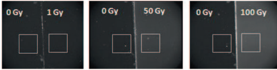
Fig. 5. – Fluorescence microscope images of an unirradiated LiF crystal (left) side by side close to an irradiated sample (right) for the LiF crystals irradiated at 1, 50, 100 Gy.
