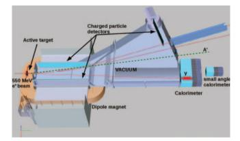
Fig. 2. – Schematics of the PADME experiment setup.
