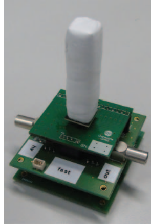
Fig. 1. – The experimental set-up based on the EJ 299-34 coupled with the Hamamatsu s13361-3050AE-04 MPPC Array. The Hamamatsu C11204-01 supplies for the bias voltage.
