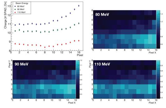
Fig. 5. – Energy released in spad-net sensor from different energies protons. (a) Top left: Charge release in number of detected photon per pixel column. At  $E_p = 80 \text{ MeV}$  there is an increase in the energy release thanks to the Bragg Peak presence; (b)–(d) Top right, bottom left and bottom right: Average energy sensor map. Each square box represent a pixel. The average number of photoelectrons detected are shown with different brightness
