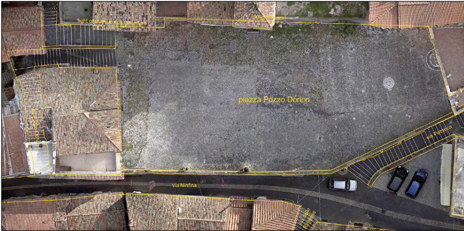
Fig. 5 – Comparison between the direct survey and the orthophotomosaic generated from aerial photographs taken by drone.
