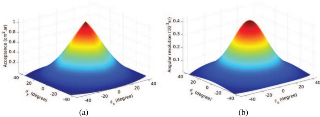
Fig. 2. – Distribution of the telescope acceptance  $\mathcal{T}$  (a) and angular resolution (b) for each discrete direction of sight of the MEV telescope ( $N = 99$ ,  $p \simeq 1.01$  cm,  $D = 97$  cm). Both quantities are displayed as functions of azimuth  $\theta_x$  and zenith angle  $\theta_y$ . The telescope axis corresponds to  $(\theta_x, \theta_y) = (0, 0)$ . The plots were created using the MATLAB software.
