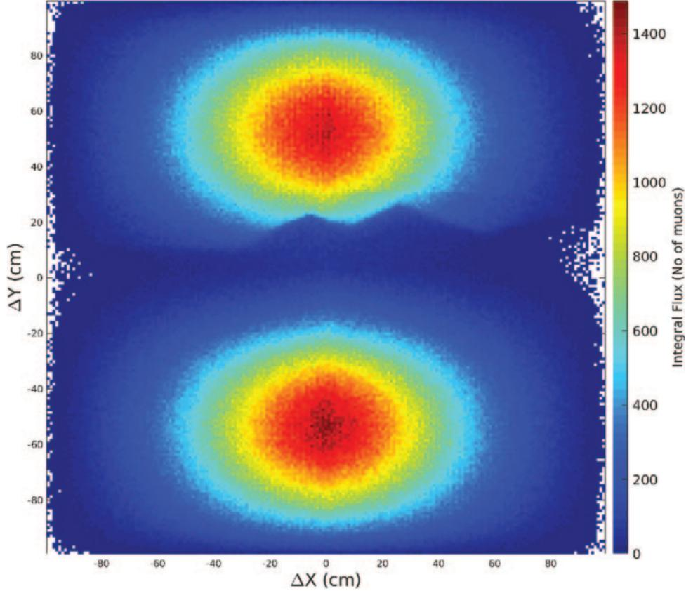
Fig. 6. – Integral of the muon flux acquired during the test phase (January-July 2017) at Nicolosi, studying the Monti Rossi. The  $\Delta X$  and  $\Delta Y$  coordinates between the crossing point of the tracks in the external planes are expressed in cm, after multiplication of  $\Delta$  in numbers of strips by strips width  $p$ .
