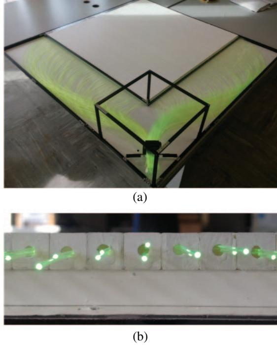
Fig. 1. – Assembly of a telescope position sensitive plane. Figure 1(a) shows on open LP with two layers of scintillation bars enclosed in an aluminum frame; fig. 1(b) is a detail of the WLS fibers embedded in each bar.
