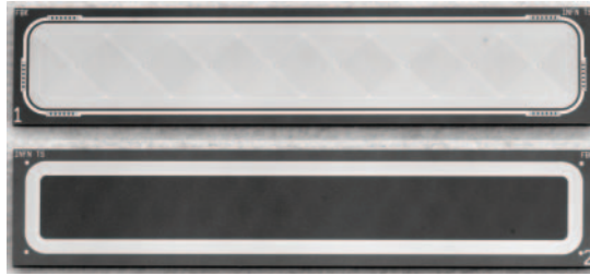
Fig. 2. – SDD linear array comprising 8 square cells with a 3 \times 3 \text{ mm}^2 active area. Anode (top) and entrance window (bottom) sides.
