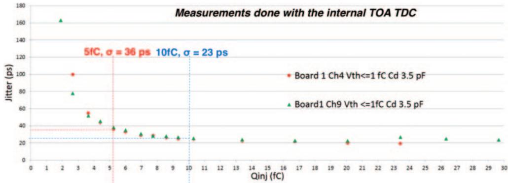
Fig. 6. – ALTIROC1 jitter measurement.
