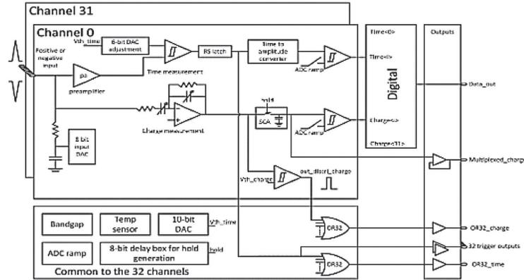
Fig. 1. – Petiroc2A block diagram.
