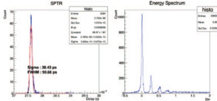
Fig. 2. – Petiroc2A SPTR with FBK NUV  $1 \times 1 \text{ mm}^2$  SiPM. The obtained value is 90.7 ps FWHM.
