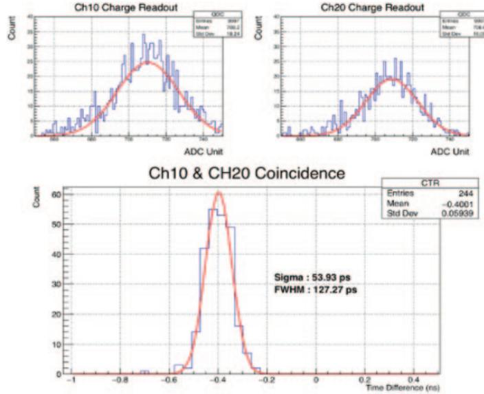
Fig. 4. – Petiroc2A CTR measured with FBK NUV-HD  $4 \times 4 \text{ mm}^2$ ,  $40 \text{ um}$  and  $2 \times 2 \times 3 \text{ mm}^3$  LSO:Ce,Ca using internal TDC. The obtained CTR value is  $127.3 \text{ ps}$  FWHM.
