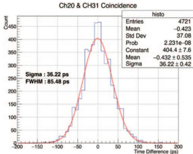
Fig. 3. – Petiroc2A CTR measured with FBK NUV-HD  $4 \times 4 \text{ mm}^2$ , 40  $\mu\text{m}$  and  $2 \times 2 \times 3 \text{ mm}^3$  LSO:Ce,Ca in analog mode. The obtained CTR value is 85.5 ps FWHM.
