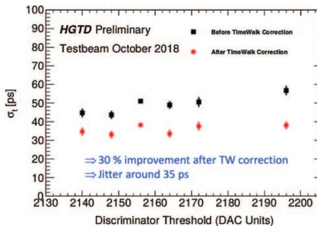
Fig. 7. – ALTIROC0 jitter measurement from testbeam.
