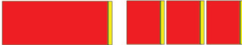
Fig. 6. – The timing error due to the timing spread in the crystal can be reduced by segmenting the gamma-ray detector.
