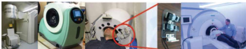
Fig. 6. – Few modern examples of the dedicated brain PET imagers. From left to right: Hamamatsu upright HiTPET imager (with patient sitting) [4,5]; the first built with SiPMs dedicated mobile brain PET; NeuroPET/CT from PhotoDiagnostic Systems (in package with CT) [3]; Cere-PET mobile brain PET with stereo-camera based motion head correction system [62-64], from Brain Biosciences; and MindView PET brain insert in 3T MRI [46,47].
