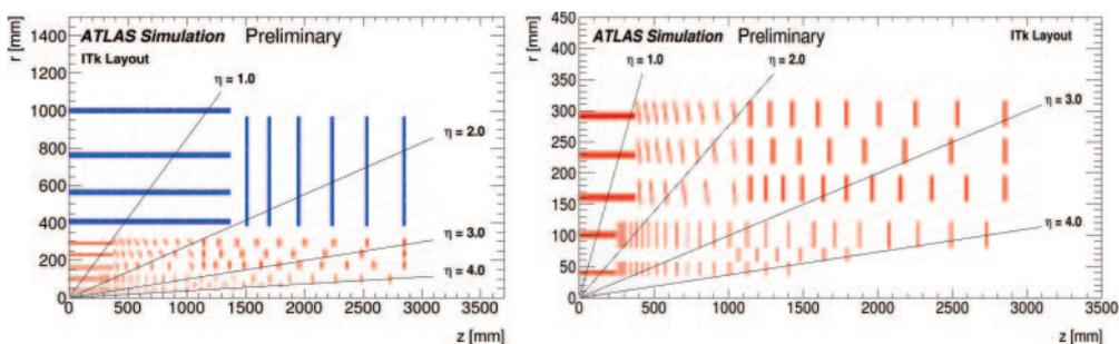
Fig. 1. – The inner tracker detector layout (left) and a focus on the pixel detector (right) [6].
