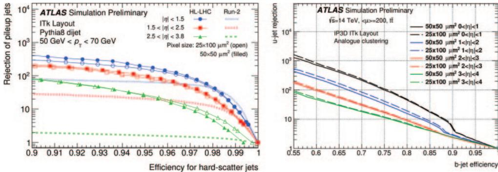
Fig. 4. – Pile-up jets rejection as a function of jet reconstruction efficiency (left) and light-jet rejection as a function of  $b$ -jet identification efficiency (right) expected for the ITk detector at the pile-up level of HL-LHC, compared to the performance of the ID at the Run 2 pile-up level. The effect of having square or rectangular pixel cells is shown as well [6].
