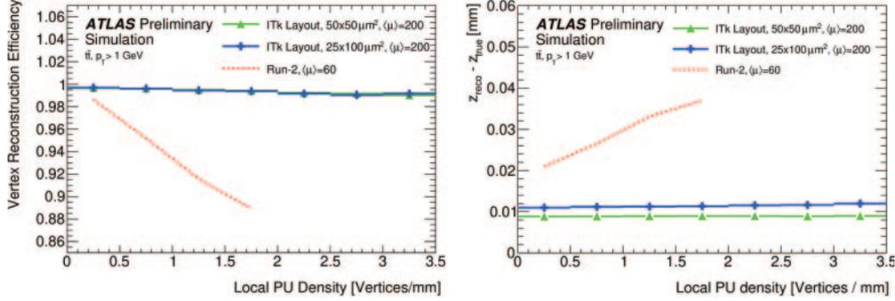
Fig. 3. – Vertex reconstruction efficiency (left) and primary vertex  $z$  coordinate resolution (right) expected for the ITk detector at the pile-up level of HL-LHC, compared to the performance of the ID at the Run 2 pile-up level. The effect of having square or rectangular pixel cells is shown as well [6].
