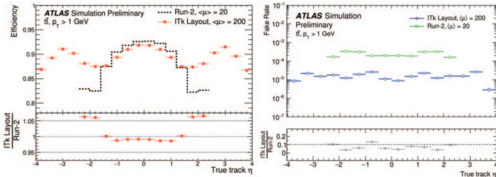
Fig. 2. – Track reconstruction efficiency (left) and fake rate (right) expected for the ITk detector at the pile-up level of HL-LHC, compared to the performance of the ID at the Run 2 pile-up level [6].
