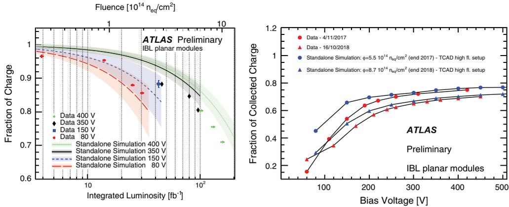
Fig. 1. – Left: charge collection efficiency as a function of luminosity. Right: charge collection efficiency as a function of bias voltage [4].
