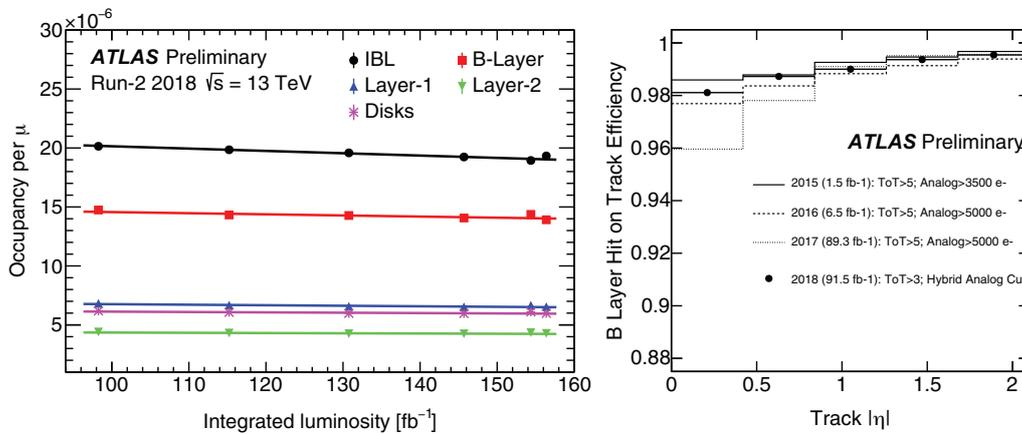
Fig. 2. – Left: the hit occupancy (the number of hits per pixel per event) per  $\mu$  as a function of the total integrated luminosity for 2018 data, for each layer of the Pixel detector [5]. Right: efficiency for B-layer hits associated to a reconstructed particle track as a function of the track pseudo rapidity  $|\eta|$  in Run 2 [6].
