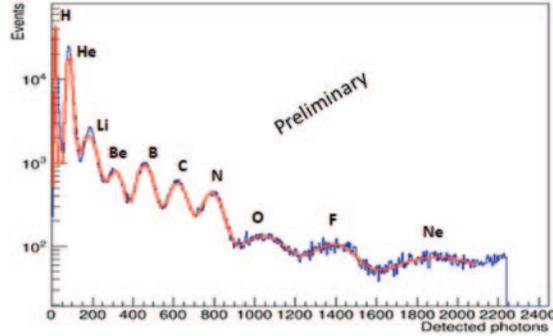
Fig. 3. – Spectrum of detected photons. The peaks corresponding to different ions have been identified performing a multi-Gaussian fit of the spectrum. These results have been obtained at the CERN SPS H4 beam line by irradiating the tile prototype in the central position [3].
