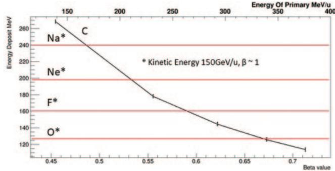
Fig. 4. – Simulation results in which the energy released by carbon ions with different  $\beta$  factors is compared with the energy released by different ions with  $\beta = 1$ .
