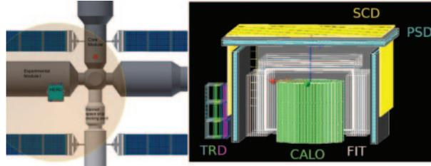
Fig. 1. – Left panel: position of the HERD facility onboard of the future Chinese Space Station (CSS). Right panel: schematic view of the HERD sub-detectors.
