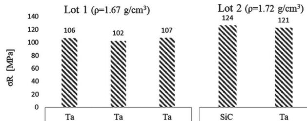
Fig. 2. – Strength data for all the cylindrical geometries at room temperature, obtained from Lot 1 and Lot 2, respectively.
