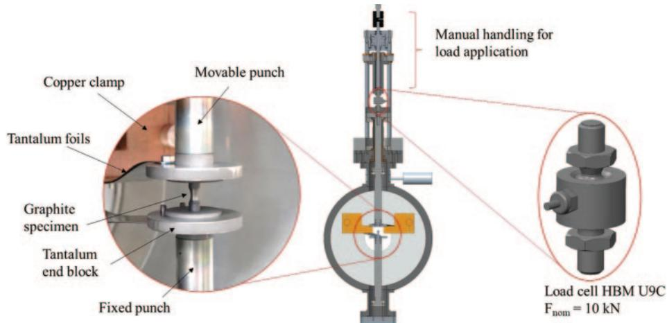
Fig. 1. – Experimental apparatus developed to apply the compressive forces for the tests.
