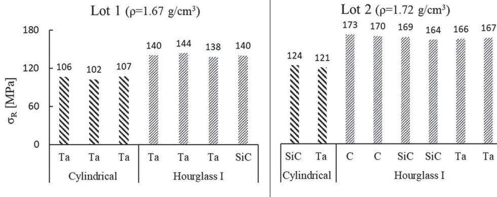
Fig. 3. – Compressive strength at room temperature for cylindrical and hourglass specimens, varying the contact material and the Lot.
