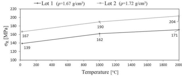
Fig. 4. – Average compressive strength with temperature in Hourglass I specimens, with lines as guides for the eye.
