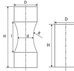
temperatures during the test. After the desired temperature was reached, the compressive test started, by applying slowly the load up to failure. The load cell allowed to obtain the compressive strength at failure.
