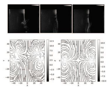
Fig. 3. – Snapshots from US imaging of MOLNBs in the magnetic field generated by four magnets in simmetric position with respect to the vertical axis. Images were recorded at different time frames (5, 15, 30 s) from the injection. Projection of magnetic fields lines in the XY and XZ plane were visualized.
