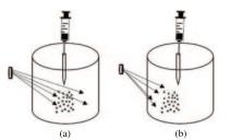
Fig. 1. – A sketch of the setup used to investigate the response of MOLNBs to magnetic fields generated by two different configurations of magnets positioned on the cylinder wall: (a) Four magnets at distance 4 cm each other in symmetric position with respect to the cylinder axis; (b) four magnets positioned in the left side of the cylinder at distance 2 cm each other.
