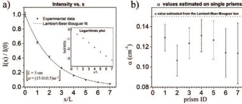
Fig. 1. – (a) Experimental data of light intensity  $I$  (normalized to  $I(0)$ ) vs.  $x$  (normalized to the prism thickness  $L$ ) inside the series of Plexiglas prisms; in the inset, the same data plot in logarithmic scale for the intensity. (b) Estimations of  $\alpha$  values through the discrete approach described in the main text; the horizontal dotted line indicates the estimation obtained with the exponential decay fit.
