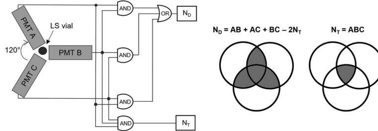
Fig. 3. – Schematic representation of the TDCR technique.
