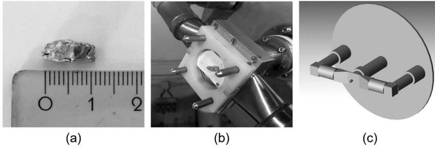
Fig. 5. – (a) Enriched  $^{64}\text{Zn}$  sample; experimental (b) and simulated (c) setup of the enriched  $^{64}\text{Zn}$  sample irradiation at the FNG facility.
