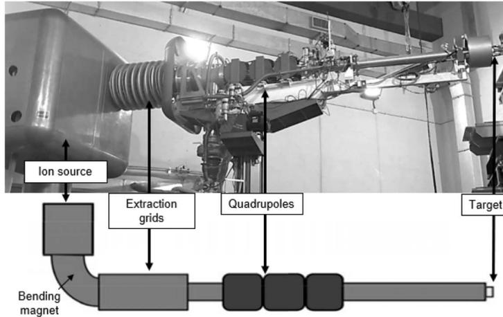
Fig. 4. – The Frascati Neutron Generator (FNG).
