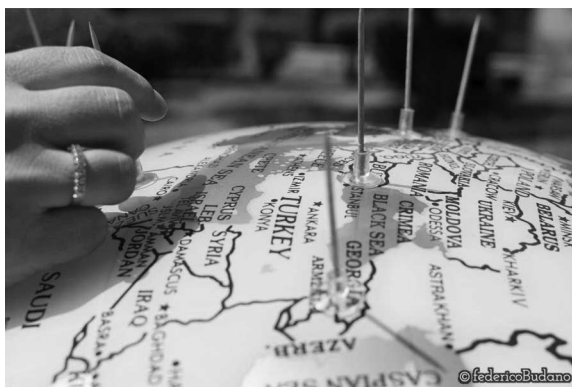
Fig. 2. – The arrangement of gnomons on the surface of the oriented globe allows us to investigate the position of the Sun in different places on the Earth as hours and days pass. Credits: Federico Budano.
